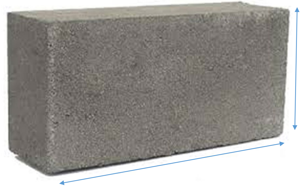
21.5cm high x 44cm long (10 blocks per m 2 inc mortar joints)
